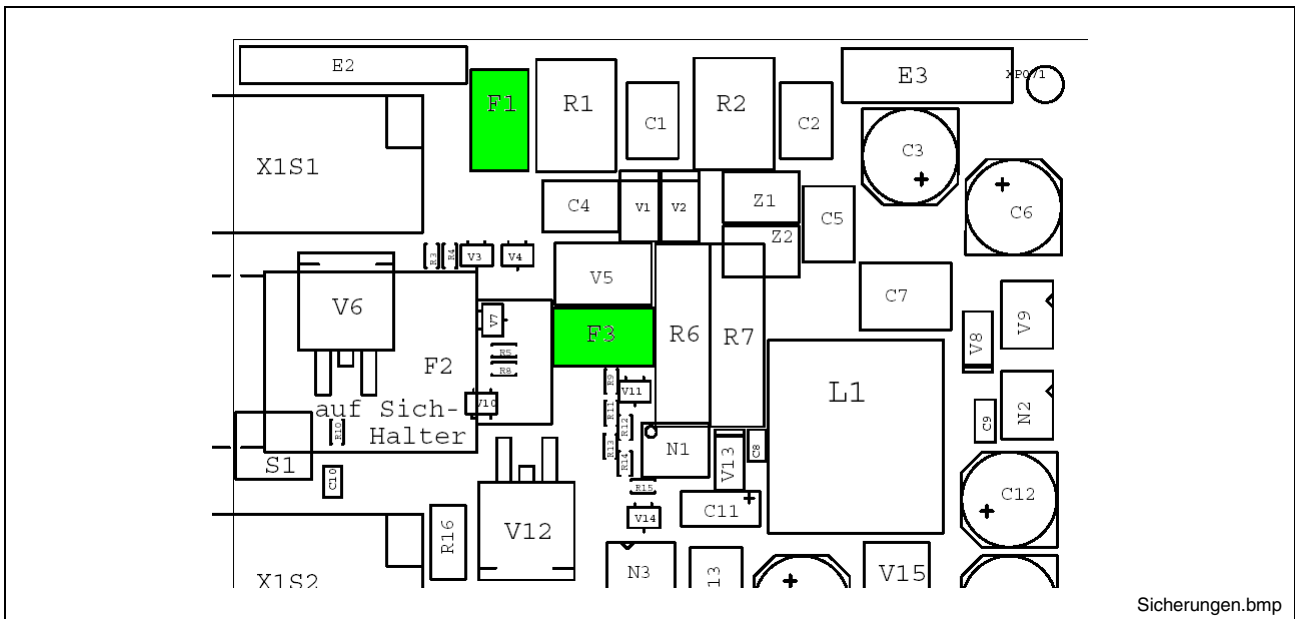
Fig. 6-10: Position of the two SMD fuses
